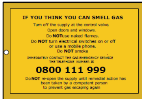
Figure 4: Natural gas emergency warning sign (Meter label)
