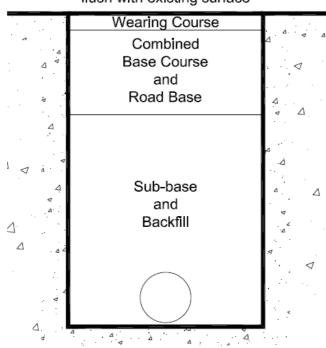
Compacted material must be flush with existing surface
